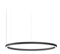
Suspension lighting fixture for interiors, with direct light emission. Bended extruded aluminium structure in white, black or mat brass polyacrylic paint. Extruded polycarbonate diffuser with opaline finish. Suspension kit with griplocks and 2m (78,7") long steel cables. 2,2m (86,6") long power cable in transparent PVC. Power canopy with pickled sheet metal ceiling bracket and covering in white polyacrylic paint.
